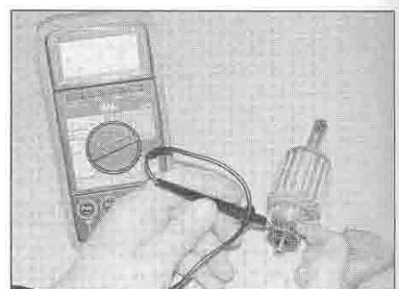
29.11 Continuity should exist between the commutator bars
