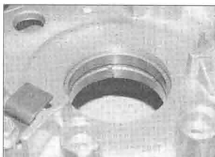
27.5 Check the main bearings as described
