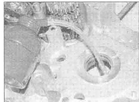
27.14 Lubricate the main bearings before installing the crankshaft
