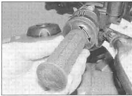
15.3 Throttle cable freeplay is measured in terms of twistgrip rotation
