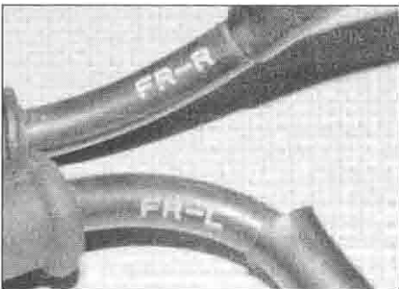
3.20 Note the markings as described and make sure all leads are correctly connected
