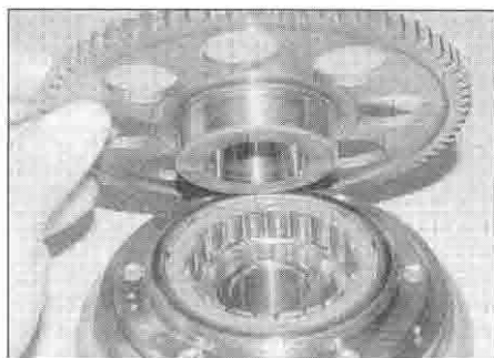
22.5a Check the condition of the sprags and gear hub as described
