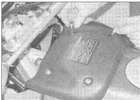
2.17a Undo the screws . . .
