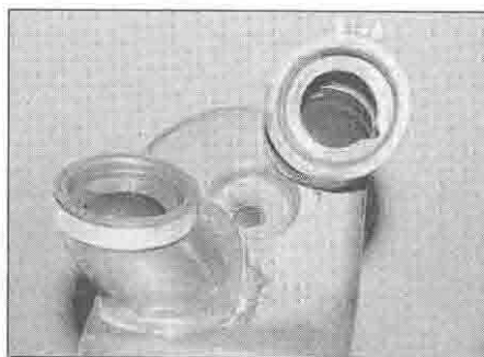
4.3b Make sure the ducts are correctly positioned
