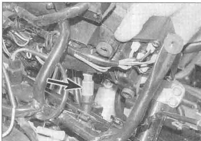
15.11c Displace the cluster and unscrew the speedometer cable retaining ring (arrowed)
