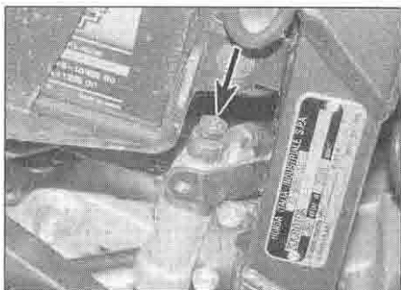
8.5 Brake hose banjo bolt (arrowed)
