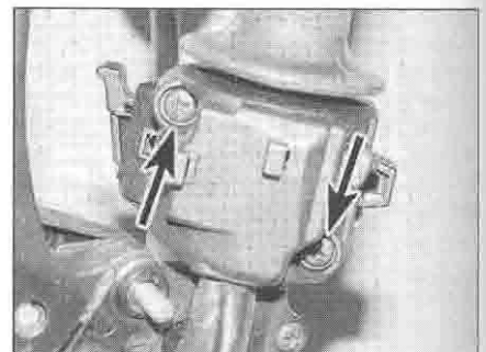
5.4b ... and left-hand switch screws (arrowed)
