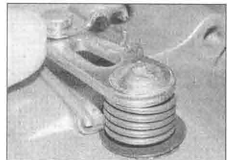
18.21d ... and the spring ends locate correctly
