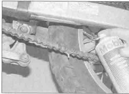
1.14 Use only the correct lubricant and apply it as described
