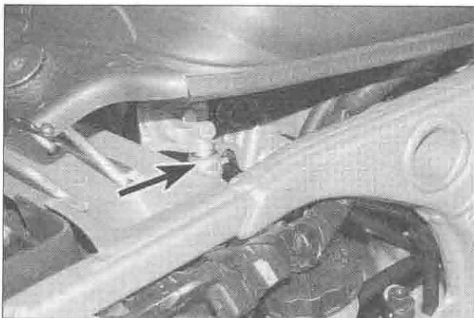
14.8a Release the clamp (arrowed) and detach the hose from the tap
