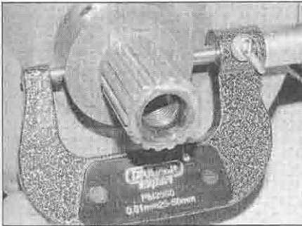
27.9a Measure the diameter of the main journal . . .
