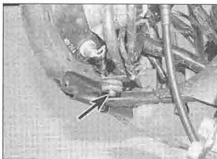
8.4e ... then lift the headlight assembly to clear the peg from the grommet
