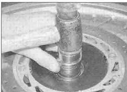
15.9 A socket can be used to drive in the bearing
