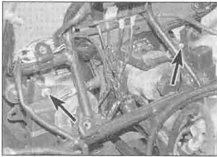
20.8b Horizontal adjustment screws (arrowed)
