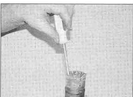
13.7a Dig out the old sealing ring ...
