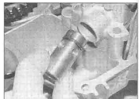
25.2c ... and withdraw the pressure relief valve
