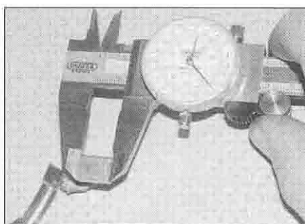
29.9 Measure the length of each brush
