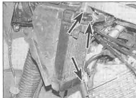
6.4b ... and the left-hand radiator – XL600V shown
