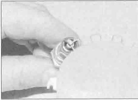
5.8a Using a wire type gauge to measure the spark plug electrode gap
