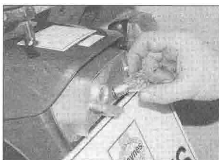
9.1c Remove the bulb as described
