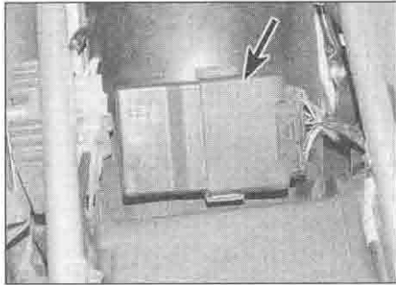
5.3a Ignition control unit (arrowed) – XL600V
