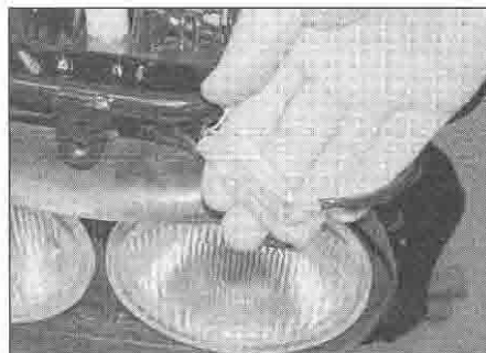
13.4 Disconnect the relevant wiring connectors ...
