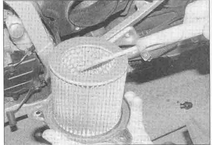
8.4 Direct the air in the opposite direction of normal flow
