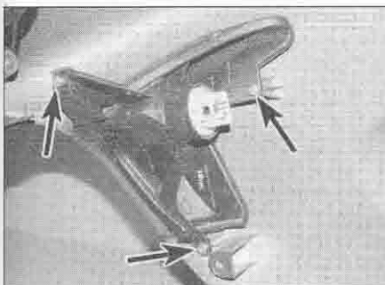
13.3b Turn signal screws (arrowed) – XL650V
