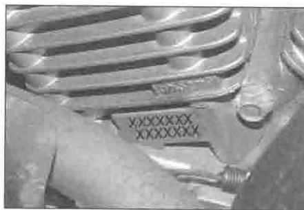
The engine number is stamped into the crankcase on the right-hand side of the engine
