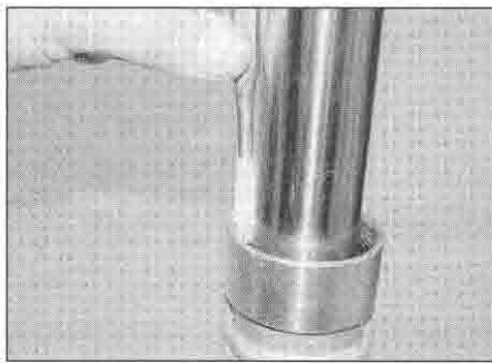
8.21c A drift can be used to tap the bush into place
