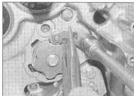
20.12b ... then position the arm on the cam and tighten the bolt
