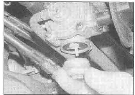
10.4b ... then thread the bowl onto the tap
