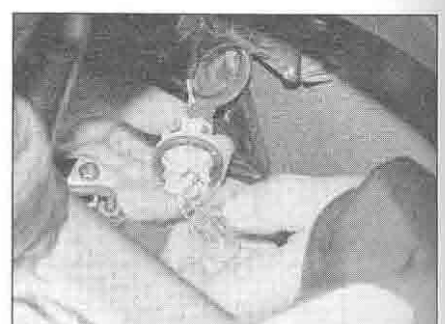
12.4d ... then pull the bulb from the holder
