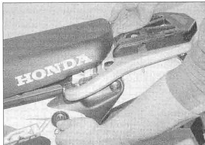
2.5a Unlock the seat, lift it up at the rear and draw it back . . .
