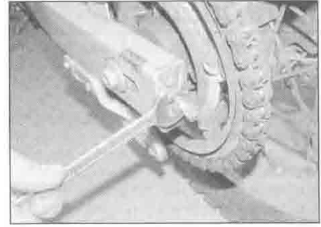
1.10b . . . and turn the adjuster as required until the slack is correct
