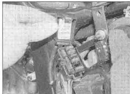
5.3e ... to access the fuses
