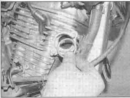
13.8 Fit a new gasket into each head
