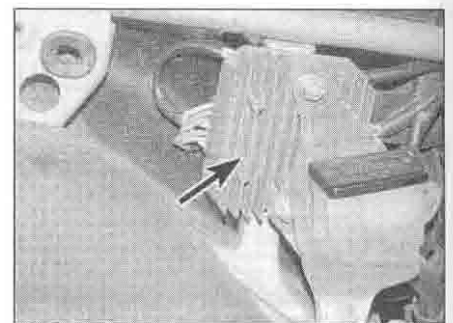
33.1a Regulator/rectifier (arrowed) – XL600V
