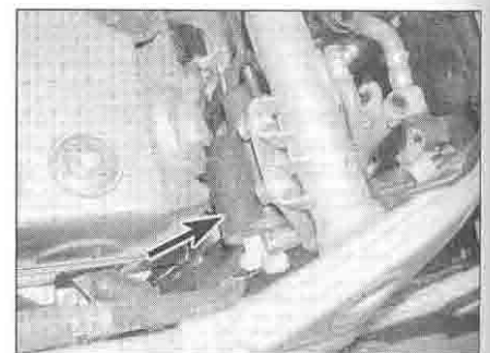
3.18e Rear cylinder HT coil (arrowed) - XRV single coil per cylinder models
