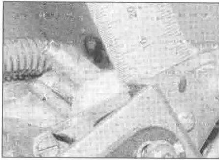
10.8 Measuring the float height
