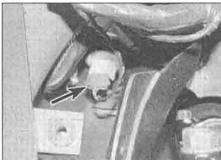
5.6 Either disconnect the wiring connector (arrowed), or release the bulbholder
