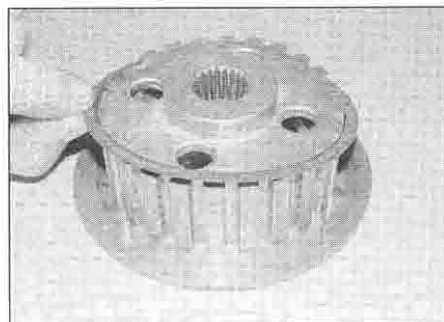
18.29a Fit the spring seat . . .
