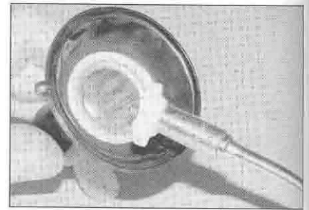
10.10 Insert the retainer, locating the spring on the top of the needle, then press down and turn to secure its tabs
