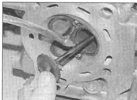
14.21b Lubricate the stem and insert the valve in the guide
