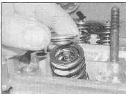
14.28c ... then fit the spring retainer
