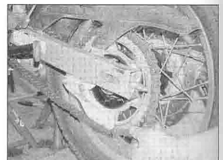
14.23b . . . then lower the wheel to the ground and disengage the chain
