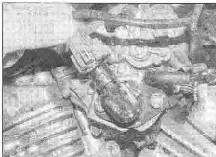
7.6a Disconnect the throttle position sensor wiring connector
