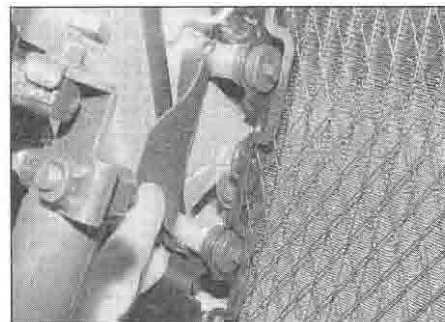
6.5c On XRV750 models move the rubber flap aside to access the bolts
