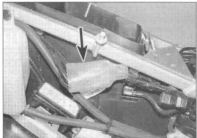
10.4 On XRV750 models the tail light and turn signal wiring connectors are inside the boot (arrowed)
