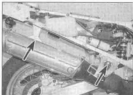
13.2f ... then unscrew the mounting bolts (arrowed) and remove the silencer
