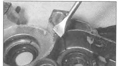
7.3 Paper gaskets can be scraped off with a gasket scraper tool ...
