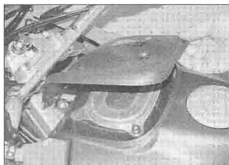
2.17b . . . and remove the cover
