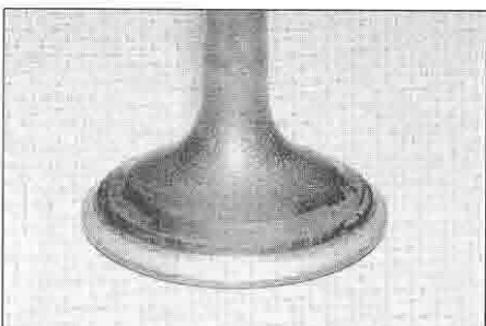
14.22b The valve face and seat should show a uniform unbroken ring and the seat should be the specified width all the way round
