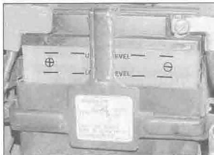
6.2 Make sure the level in each cell is between the UPPER and LOWER level lines
