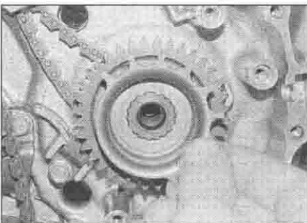
21.8 ... and on XL models the timing rotor
