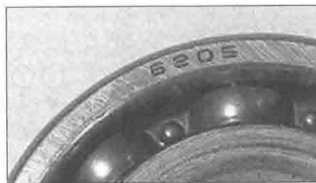
5.16 Typical bearing marking
