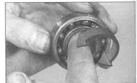
5.19 Hold outer race and listen to inner race when spun
