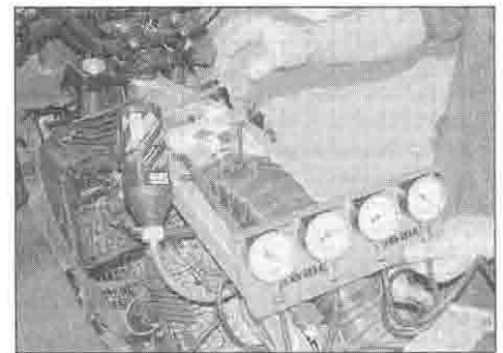
17.11 Adjusting carburettor synchronisation. Note how on XL models the adjustment screw is accessed via the hole in the air duct or filter housing
