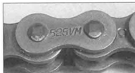
8.10 Typical chain size and type marking
