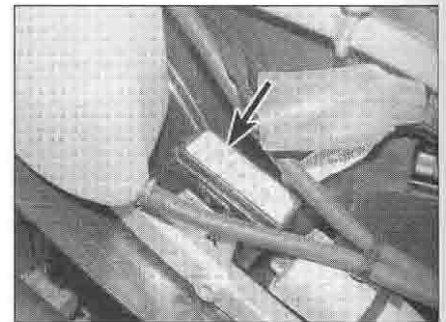
5.3c Fusebox (arrowed) – XRV750-P models on
