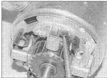
29.17 Locate the spring ends onto the brushes
