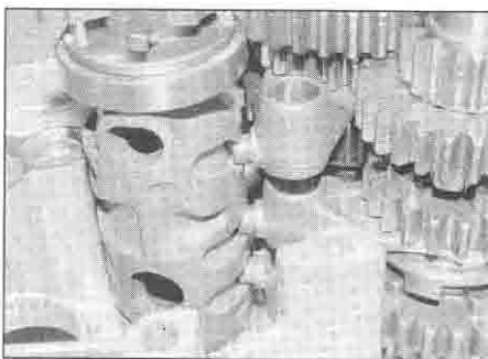
29.27 Pivot each fork so its guide pin locates in its track in the drum
